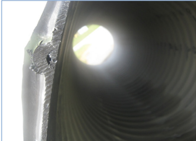
Figure 1: 5 mm diameter channel on exterior of HDPE pipe
