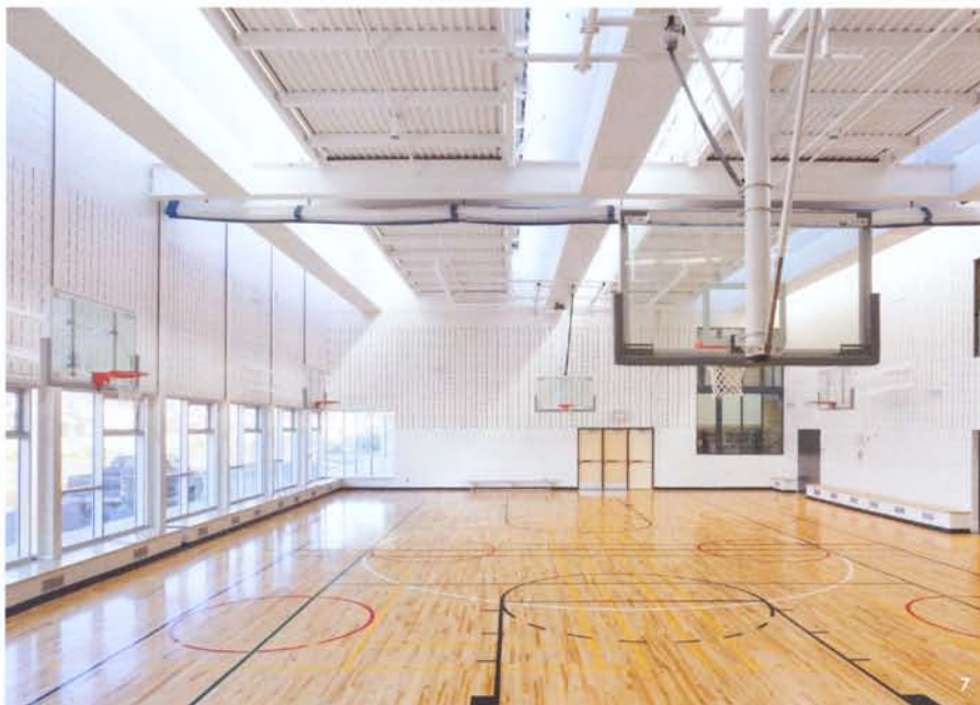
NATURAL "TOP-LIGHT" DAYLIGHTING AND VENTILATION PARTLY SERVICE THE GYMNASIUM, WHICH ALSO DOUBLES AS A MULTI-PURPOSE ROOM [7].
